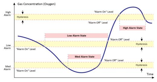
Alarm hierarchy exists. An A2 alarm overrides an A1 alarm on the display. However, the A1 and A2 states operate independently. An example follows.
