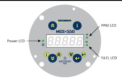
After the warm-up period, the instrument begins normal operation. The display toggles between the current gas concentration and target gas name.
